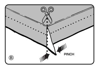
© Fold the fabric to the underside, again pinch and trim. A few staples in the underside will ensure the fabric is held in place whilst the adhesive cures.
