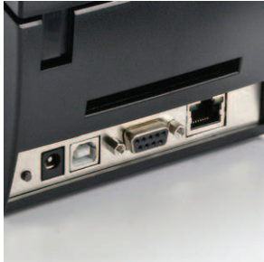
Ethernet, Serial and USB are standard features adding flexibility and power
