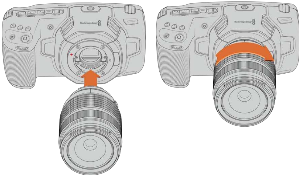
Attaching an MFT lens on Blackmagic Pocket Cinema Camera 4K
