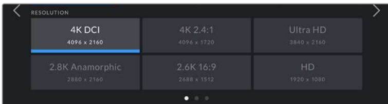
Pocket Cinema Camera 4K 'resolution' options. Note that in 4K DCI format the category is 'resolution', otherwise it's 'resolution - sensor windowed'.
