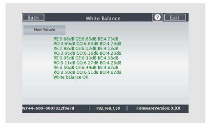
$oldsymbol{0}$  On an error-free white balance calibration, the result is displayed in green.
