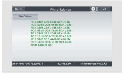
On an error-free white balance calibration, the result is displayed in green.
