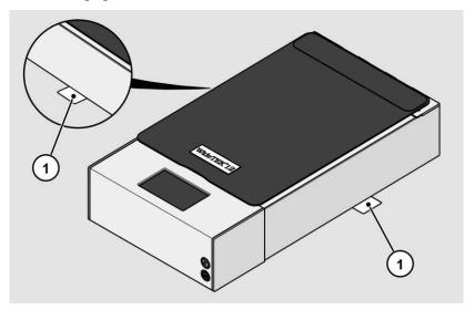
You must remove the transport locks before using the scanner for the first time. To remove the transport locks, proceed as follows:
