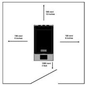
Place the WideTEK® 12 or WideTEK® 25 scanner on a flat and solid base. The load bearing capacity of the base must correspond to the device weight. The dimensions of the base must match the floor space required by the scanner.
