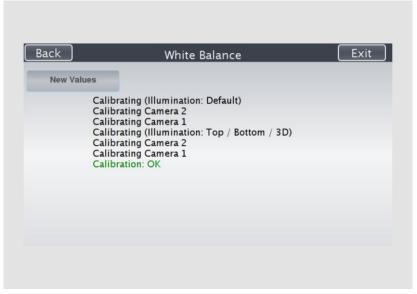
$\ensuremath{\bigcirc}$  On an error-free white balance calibration, the result is displayed in green.
