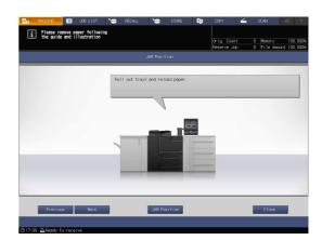
4 Remove all jammed paper, then press [Close]. This returns to the [MACHINE] screen.
