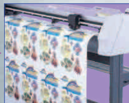
Contour cutting by the CG-FXII series
