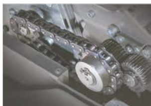
SUPER POTENTIAL POWER SYSTEM: chain drive system with steel gears.
