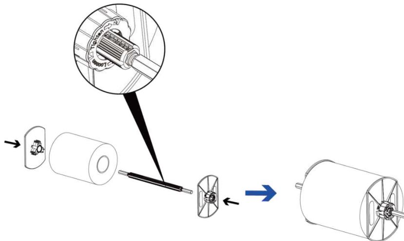
Step 3. Put the label roll into label roll stand.
