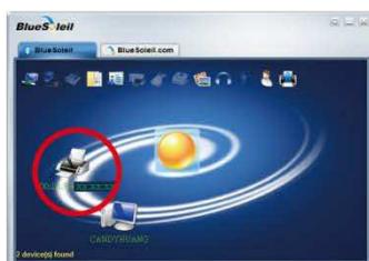
Step 6. Right-click on the mouse and select "Get Device Name" and the icon of the printer will display "HD830i"
