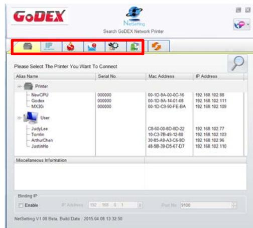
**Step.02** ➔ There are six tabs on the top of interface which can configure different types of network settings. But for the data security reason, you need correct password to enter the configuration pages.
