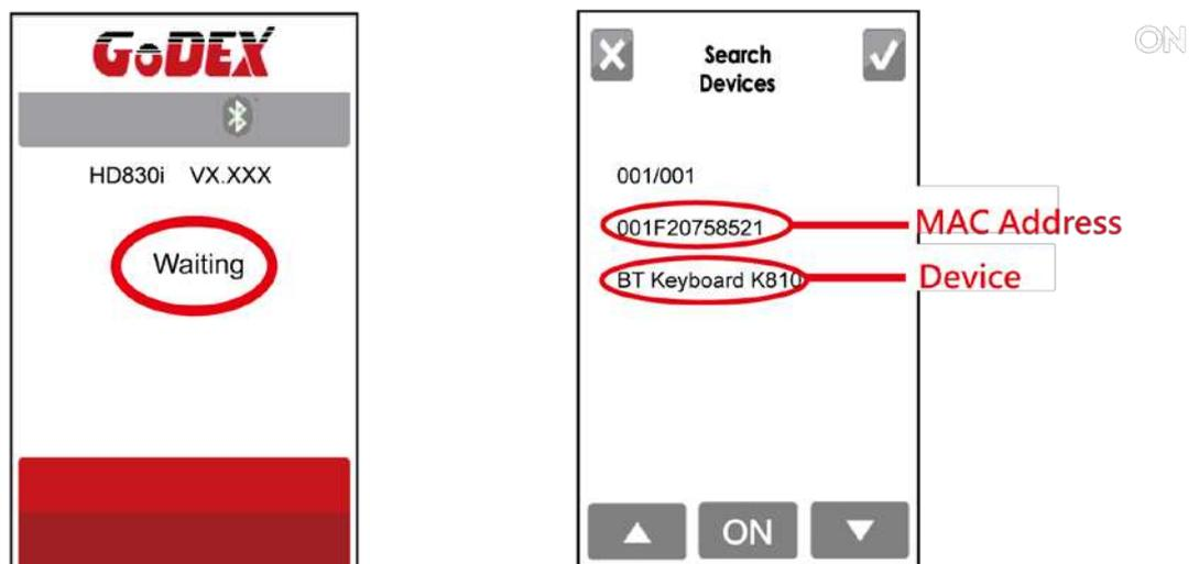
Step 7 . Press "ON" button on the LED panel to create a connection between the printer and the Bluetooth keyboard, and then the LCD panel will display " Please Enter PIN Code " .
