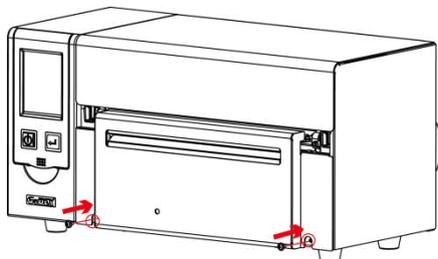
Step 4. Fasten the screw in position.
