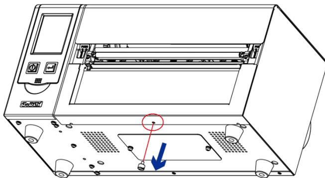
Step 1. Disassemble the bottom case screws (Marked in Red circle)
