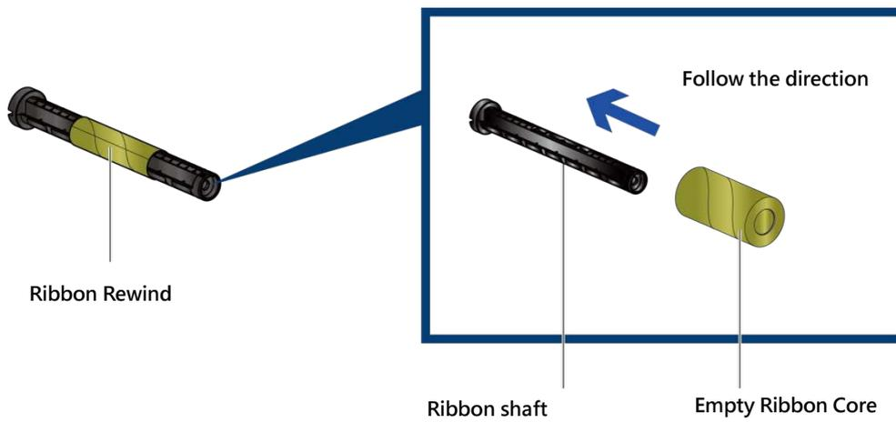
Stick the ribbon with the Ribbon Rewind units and rolling 2~3 cycles.
