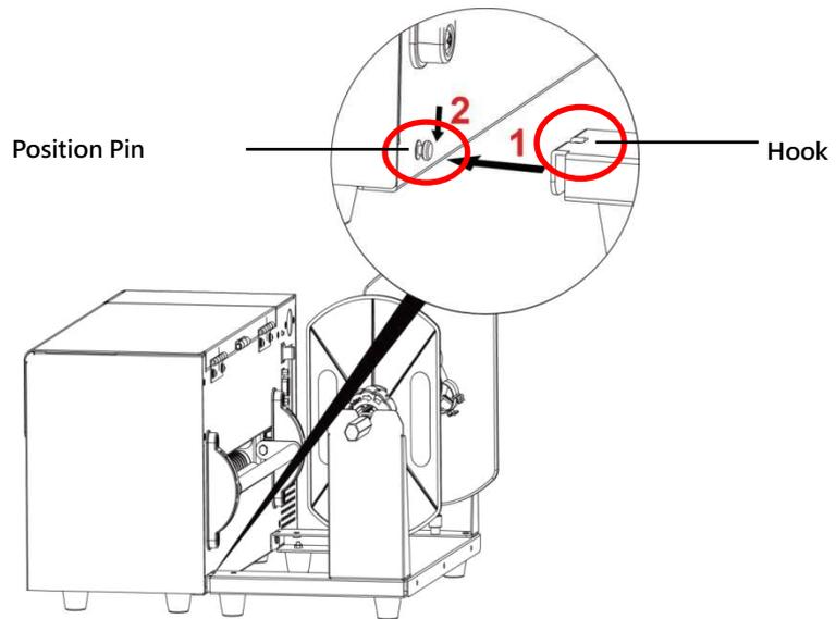
Step 2. Following the below arrow mark and direction to put the label roll into position.
