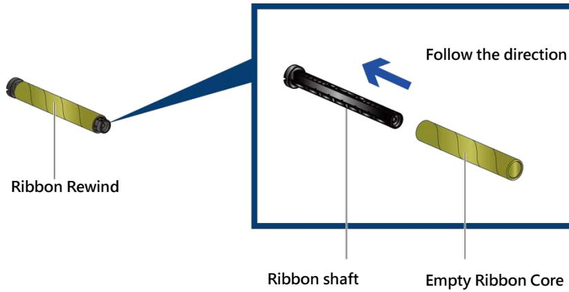
Stick the ribbon with the Ribbon Rewind units and rolling 2~3 cycles
