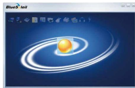
Step 3. Select the desired icon with the mouse and right-click on the mouse to select " Turn on Bluetooth" (The Bluetooth device now lights up in green.)
