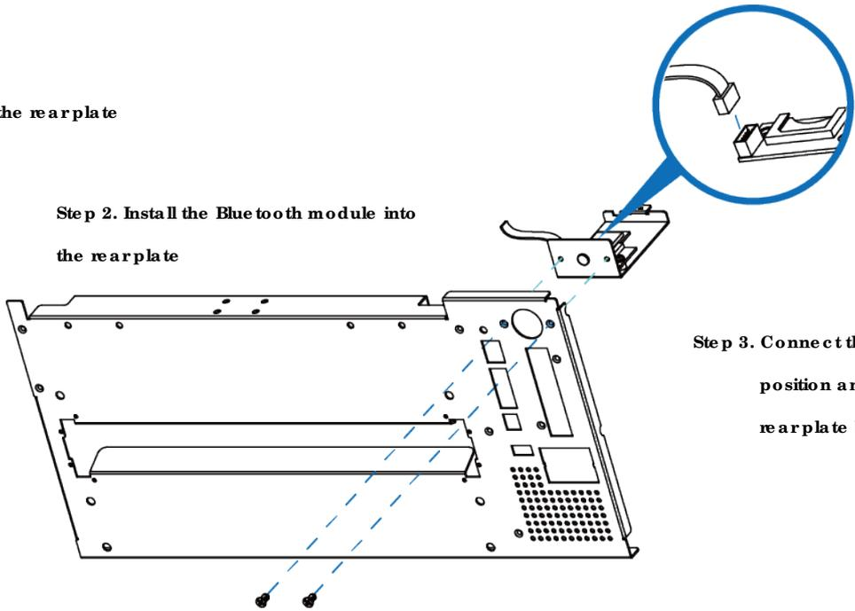
Step 3. Connect the cable into position and fasten the rear plate back to printer
