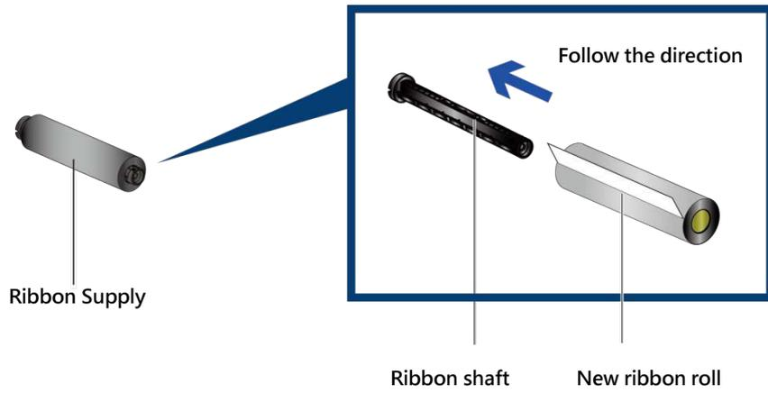
Install the empty ribbon core into ribbon shaft
