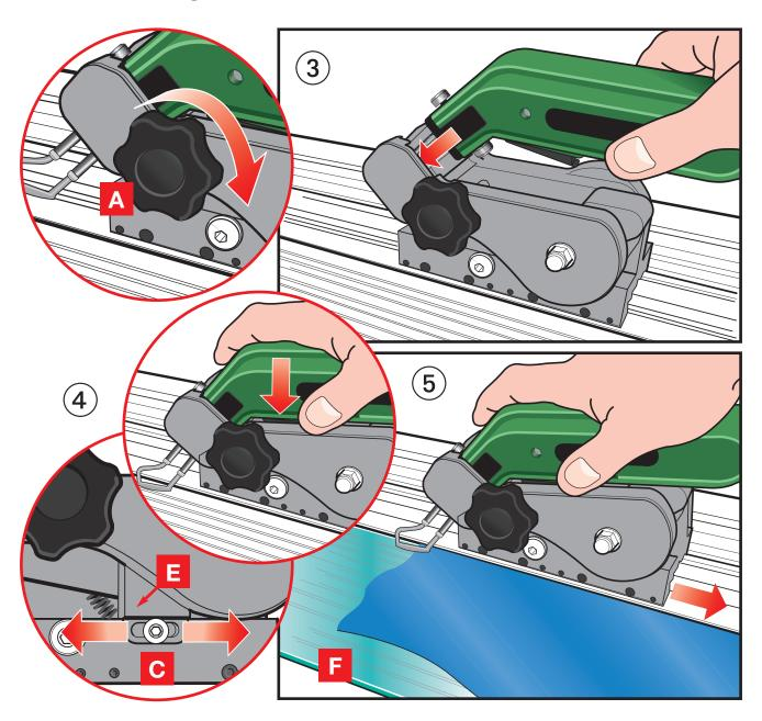
3 To fit the Hot Knife, simply insert it into the holder ensuring the nose of the Hot Knife is seated fully into its recess.
