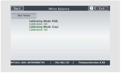
$\bigcirc$  On an error-free white balance calibration, the result is displayed in green.
