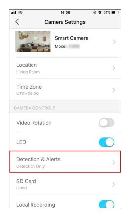
2. On the Detection & Alerts page, enable the Motion Detection function. It's recommended to enable the Notifications function to receive motion detection messages.
