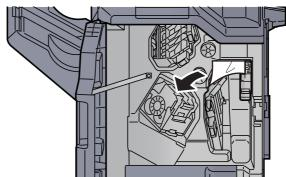
Q Return the conveyor guide (D1) to the original position.
