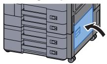
If the optional side feeder is installed, return the side feeder to the original position.
