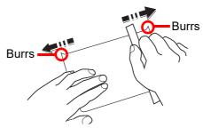
Before loading Hagaki (Cardstock), fan them and align the edges. Hagaki (Cardstock) should be fed from the multipurpose tray with the print-side down or the cassette and the optional paper feeder with the print-side up. If the Hagaki (Cardstock) paper is curled, straighten it before loading. Printing onto curled Hagaki (Cardstock) may cause jams.
