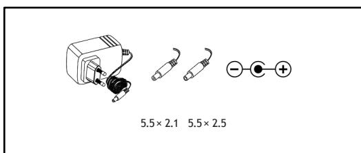
4 batteries type C (LR14) or AC adapter.
